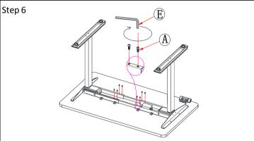
Tighten Crossbeams (part 4) using (part A) Screw M6x10.
