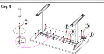
Adjust Crossbeams to the proper position to fit the desktop. Tighten the (part C) Wood screw ST4.8x19 to lock. Attach the Handset (part J) and Control box (part H) to the underside of the desktop using (part D) Wood screw ST4.2x16.
