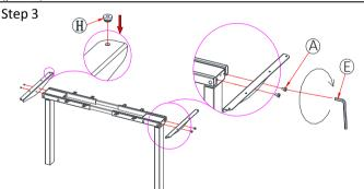
Attach the Side bracket (part 3) to the Crossbeam (part 4) using (part A) Screw M6x10. Rubber gasket (part G) into the hole on the Side bracket (part 3) and the Crossbeam (part 4).
