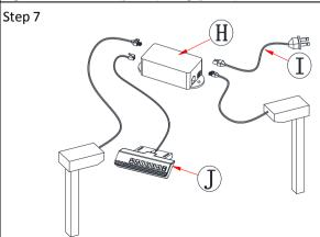
Connect the Lifting legs (part 2), Handset (part J), and the Power cable (part I) to the Control box (part H).
