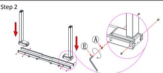
Attach the Lifting leg (part 2) to the Crossbeam (part 4) using (part A) Screw M6x10.
