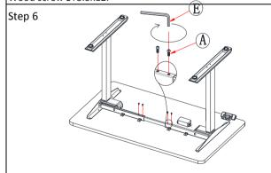
Tighten Crossbeams (part 4) using (part A) Screw M6x10.
