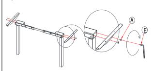
Attach the Side bracket (part 3) to the Crossbeam (part 4) using (part A) Screw M6x10.
