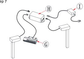
Connect the Lifting legs (part 2), Handset (part G), and the Power cable (part I) to the Control box (part H).
