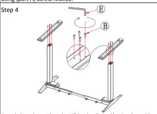
Attach Foot (part 1) to the Lifting leg (part 2) using (part B) Screw M6x16.
